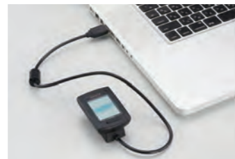
USB cradle for battery recharge and data upload
